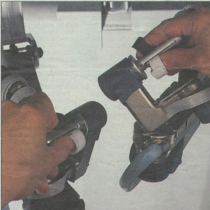
**REMOTE CONTROL:** By sitting at a console away from the patient, the surgeon can work the robot as if it was an extension of his hands. The machine will copy his movements but the degree of movement can be broadened or shortened to control a fiddly area.
